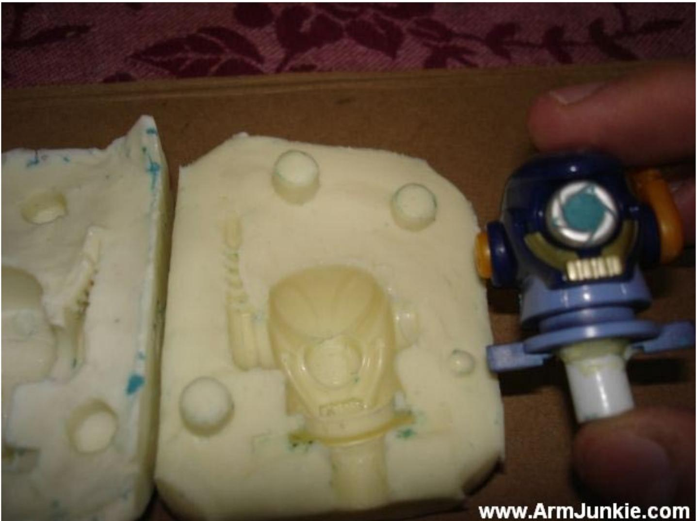
In this image, you can see the pour channel used for pouring the plastic resin into the mold cavity.
