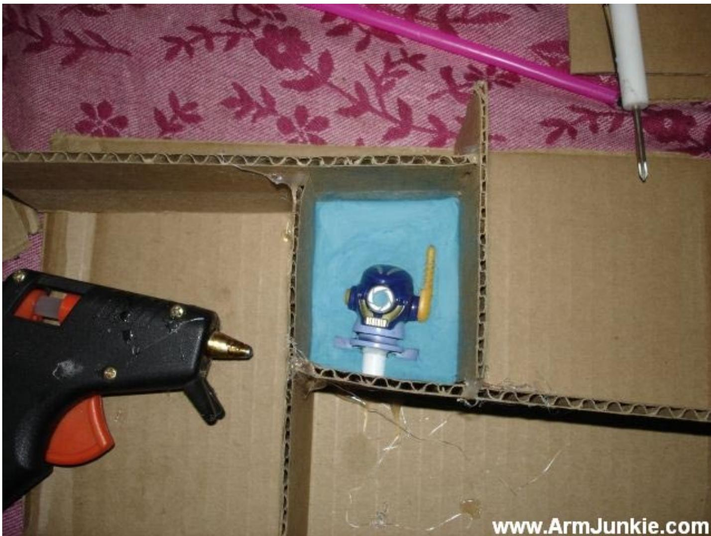
The clay must be as smooth as possible. Take special care to cover up any exposed edges around the object. Press in the eraser end of the pencil into the clay a few times. This will dimple the clay, making two interlocking pieces.
