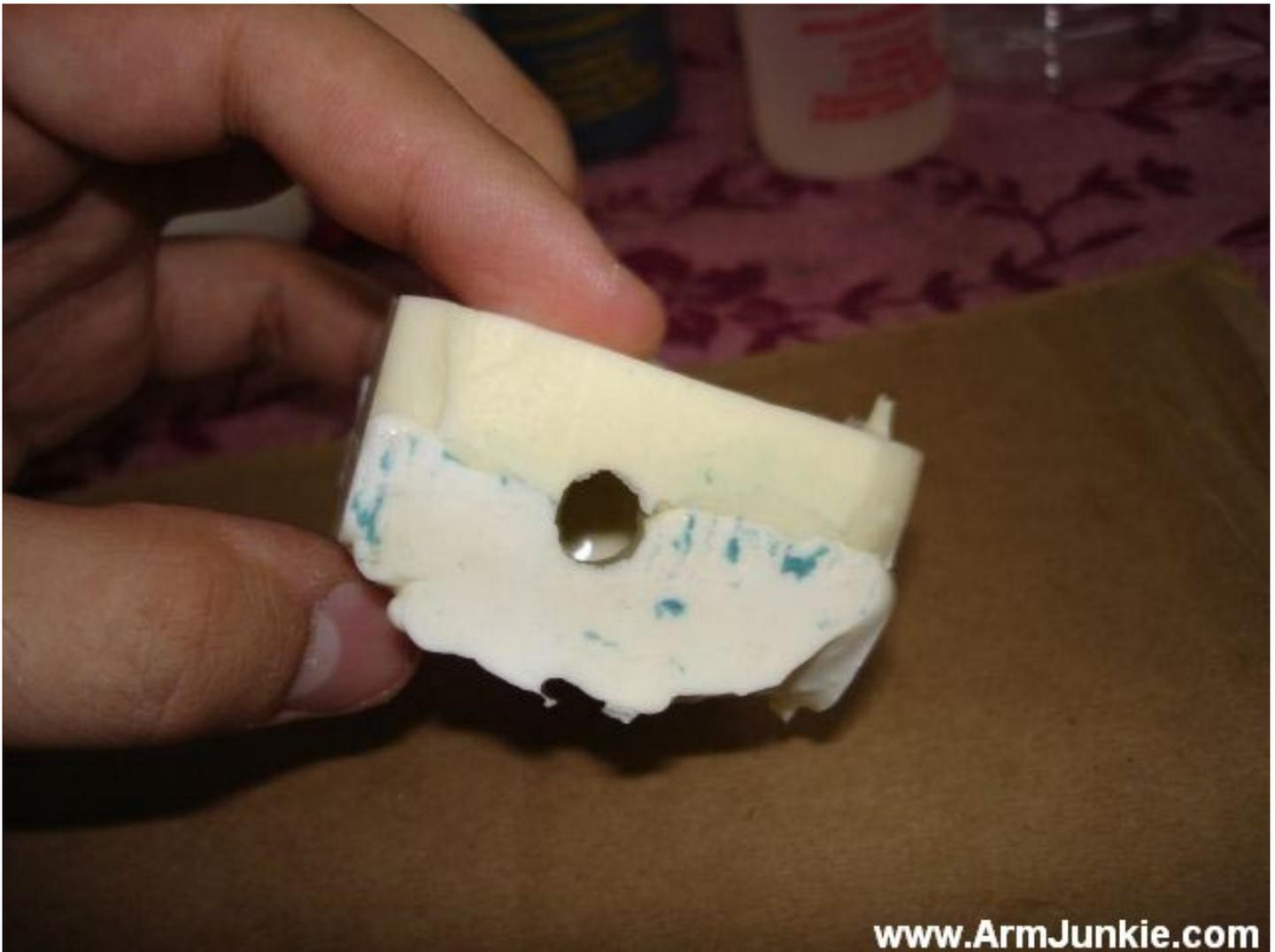
All things considered, it's a pretty good mold for a first timer. I can see that the mold won't be perfect. I got some air bubbles trapped due to not having my own vacuum chamber. I can see a problem with the robot's antenna. It must have moved during the mold making process. It doesn't look like the antenna will cast properly but let's continue anyway.
