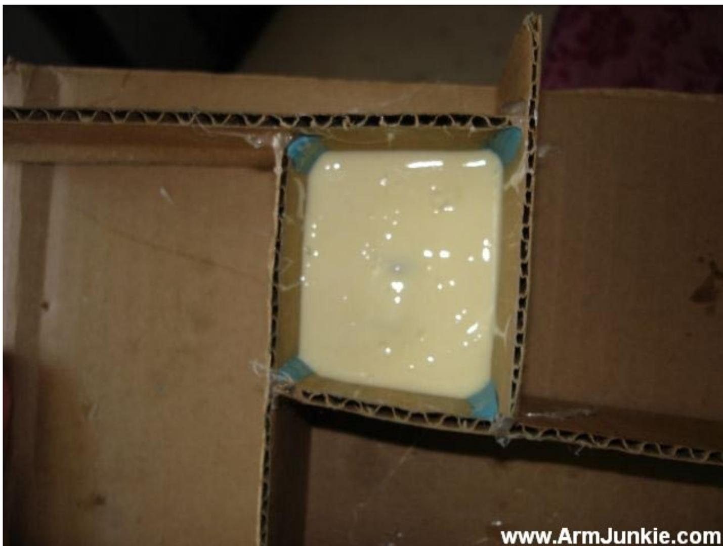
Once the silicone has hardened I removed the back of the cardboard mold. I carefully picked off the clay. Here is where I made my first huge mistake. I got overexcited and decided to remove the robot head to take a picture. This was a huge mistake because once dislodged, the piece would no longer fit snugly when placed back. This will produce a slightly warped piece and the “antenna” on the side will be completely ruined.
