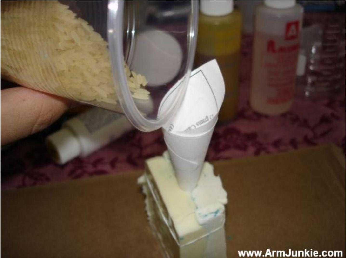
Here the mold cavity is filled with rice. Pour out this rice into a measuring cup to find out the volume of the cavity. It's a good idea to give yourself a nice buffer because a little over spilling is better than under filling.
