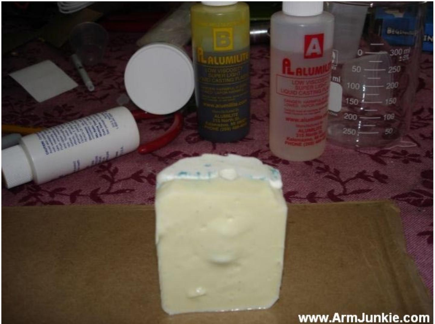
You can clearly observe the color difference between the two silicone mold halves. This is more proof that my chemicals are old and that I failed to do proper, even mixing. The silicone chemical was not uniformly mixed. Pouring the second batch of silicone was even more difficult and took longer to dry and harden. It's amazing that anything was cast at all.
