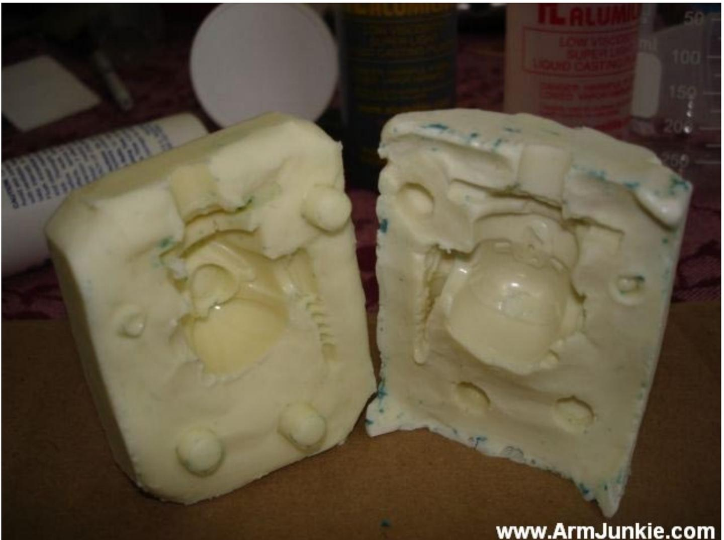
Notice how dimpling one side in the clay produced the interlocking teeth. Other than the botched antenna there were no serious mold deformations. You can spot two small air bubbles on the left edge of the left mold half in the following image.
